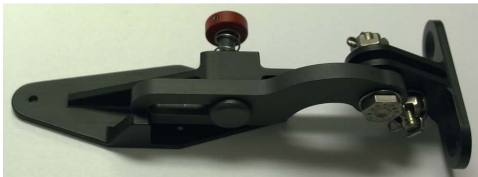
Figure 3.2: Hinge, Locking Assembly (Baggage Compartment Door in Open Position)
